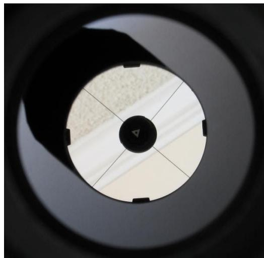
**Figure 3:** View of a perfect collimated Newtonian telescope.
